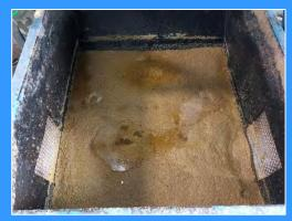
Hops, Yeast, Trub and CIP waste stream filtered and converted to energy rich sludge cake.
